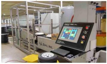
exception of the inflation heads which are changed to match rim sizes. Inflation pressure is set and can be maintained up to +/- 1 PSI. Production logging and recipe storage are also available as options. Remote system maintenance via the internet is also available if the customer requires it.
