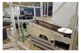
An unloading system at the end of the conveyor strips the inflated wheel assemblies from the indexing conveyor and deposits them on a gravity conveyor. A photo eye on the gravity conveyor stops the system if the gravity conveyor is full. The Conveyor system can be specified or set to any length that the customer desires.
