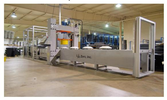
L/A Wheel System's Automatic Tire Inflator that can inflate wheel assemblies ranging from 12" diameter to 32" with speeds up to 600 wheels per hour in continuous mode,
